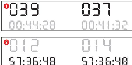
The lap counter recognizes a vehicle when it passes through the light barrier. Lap races ① or time trials ② can be executed. Here you can set a maximum of 999 laps, or 59 minutes and 59 seconds.
